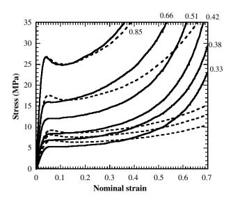
Fig. 12. Compression tests for different relative density foams. The values on the curves represents the relative density. The dash lines represents the predicted values with the secant modelling. Initial strain rate =  $10^{-3}$  s<sup>-1</sup>, T = 30 °C.
