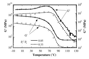
Fig. 7. Evolution of elastic modulus (G') and loss modulus (G'') as a function of temperature obtained by DMA. The values on the curves represents the relative density. The circles represents the predicted values with the 2 + 1 phase modelling. f = 0.1 Hz, T = -10 up to 130 °C, dT/dt = 1 °C/min.
