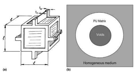
Fig. 11. (a) Cubic cell used for the Gibson and Ashby modelling [1] of closed cells foams. The cell is constituted of struts (length l, thickness  $t_e$ ) and walls (thickness  $t_l$ ). (b) schematic representative volume element used in the 2 + 1 phase modelling.
