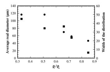
Fig. 6. Average real diameter (square) and distribution width (circle) of the cells of foams as a function of relative density.
