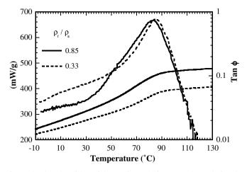
Fig. 3. Analyse by differential scanning calorimetry and DMA for the different foams processed. The values on the curves represent the relative density. T = -10 up to 130 °C, dT/dt = 10 °C/min for test by DSC. f = 0.1 Hz, T = -10 à 130 °C,  $\Delta T = 1$  °C/min for test by DMA.
