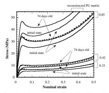
Fig. 2. Compression curves of polyurethane matrix and foams with different aging stages. The values on the curves represent the relative density. The polyurethane matrix curves are calculated from the dilute sphere and the high density foam ( $\rho_{\rm f}/\rho_{\rm s} = 0.85$ ). The dash lines represents the simulated values. Initial strain rate =  $10^{-3}$  s<sup>-1</sup>, T = 30 °C.
