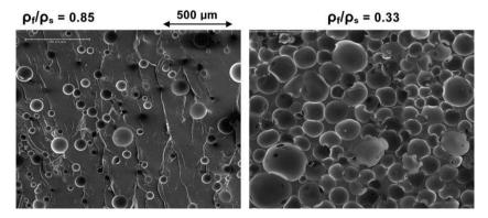
Fig. 4. SEM micrographs of foams.
