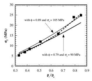
Fig. 10. Evolution of the stress value at the beginning of the plateau ( $\sigma^*$ ) as a function of relative density obtained by compression tests. The lines represents the predicted values with the Gibson and Ashby modelling [1]. The dash line represents the predicted values with the phenomenological modelling. Initial strain rate =  $10^{-3}$  s<sup>-1</sup>, T = 30 °C.
