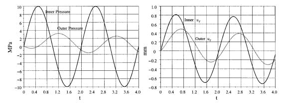
Figure 2. Time evolution of pore pressure and radial displacement on the inner and outer surface of the hollow sphere (first example).
