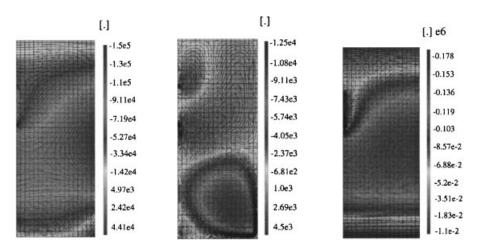
Figure 7. Corresponding contour of  $\delta_M \sigma_{zz}$ ,  $\delta_M \sigma_{rz}$ ,  $\delta_M p$  at the middle of the transient phase (axisymmetrical modelling, second example).
