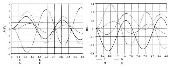
Figure 3. Time evolution of the sensitivities coefficient of the outer pore pressure (left panel) and of the radial displacement (right panel)  $(m_i \delta_{m_i} u_r (r = R_e, t))$  for the hollow sphere (first example).
