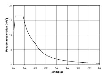
Fig. 3. 20% damped bedrock response spectrum.
