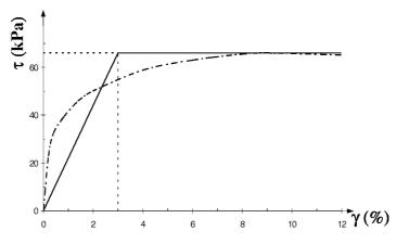
Fig. 2. Soil shear stress-shear strain curve.
