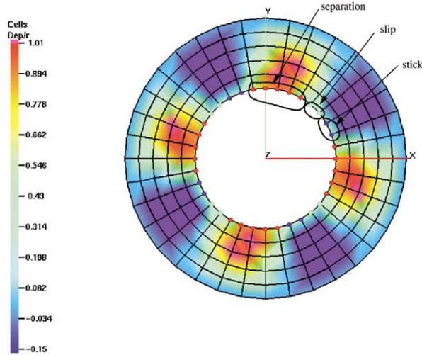
Fig. 5. A mode-4 stick–slip–separation wave, obtained by numerical simulations for  $\xi = 2$ ,  $\Omega = 50$  rad/s,  $f = 0.7$ ,  $\delta = 0.001$ . The isovalues of the radial displacement (mm): separation, slip and stick nodes on the contact surface are given respectively in red, green, blue.
