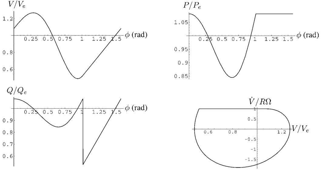
Fig. 4. Semi-analytical approach: an example of stick–slip wave in mode 4 with  $\xi = 2$ ,  $f = 0.3$ ,  $\Omega = 10$  rad/s,  $R = 0.25$  m and  $\delta = 0.005$ . It is found that  $\Psi = 0.644$ ,  $c = 1030$  m/s. Phase diagram and variations of  $V/V_e$ ,  $P/P_e$  and  $Q/Q_e$  in  $[0, 2\pi/k]$ .
