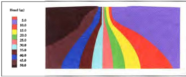
Figure 8. Head contours calculated with the identified permeabilities.
