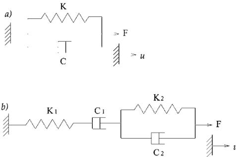
Fig. 2. The Kelvin-Voigt model, and the four-element model.
