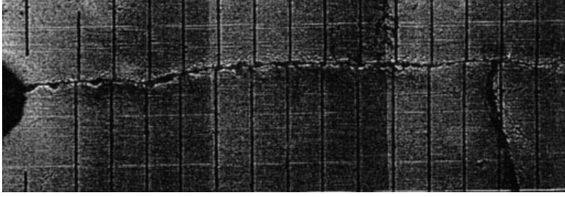
Fig. 1 Branching of a mode II crack from a crack flank in a maraging steel (the distance between engraved lines is 100 \mu\text{m} ).
