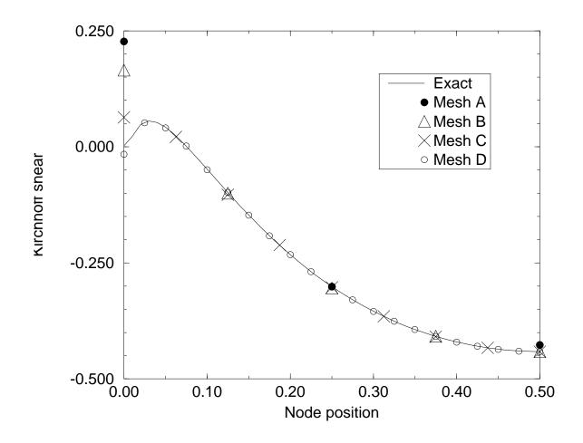
Figure 2: Clamped plate: Kirchhoff shear.
