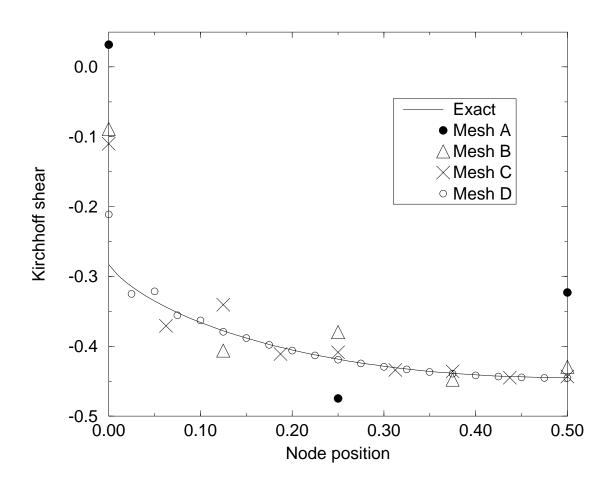
Figure 7: Simply-supported-free plate: Kirchhoff shear along a simply-supported side (3-noded interpolation).
