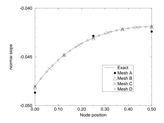
Figure 6: Simply-supported-free plate: normal slope along a simply-supported side.
