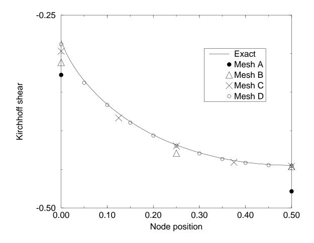
Figure 8: Simply-supported-free plate: Kirchhoff shear along a simply-supported side (2-noded interpolation).
