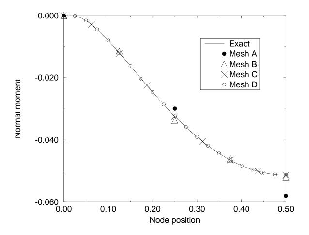
Figure 1: Clamped plate: normal moment.
