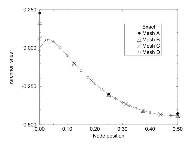
Figure 2: Clamped plate: Kirchhoff shear.
