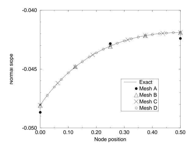
Figure 6: Simply-supported-free plate: normal slope along a simply-supported side.
