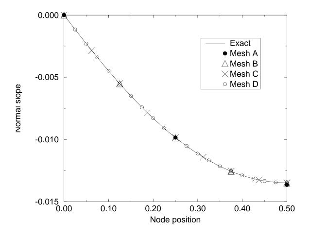
Figure 3: Simply-supported plate: normal slope.
