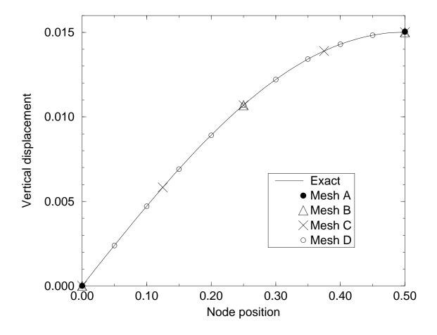
Figure 5: Simply-supported-free plate: vertical displacement along a free side.
