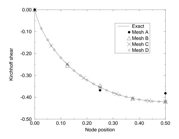
Figure 4: Simply-supported plate: Kirchhoff shear.
