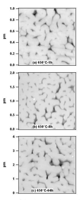
Fig. 3. AFM height images of three borosilicate glass samples. These images illustrate the similarity of morphology of the phase separation domains for various observation scales according to the duration of thermal treatment at  $650^{\circ}$ C.
