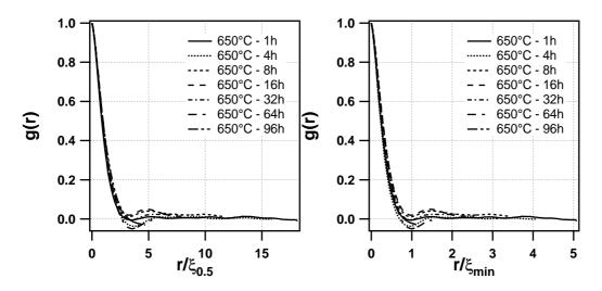
Fig. 8. Radial mean value of the auto-correlation function  $(g(\mathbf{r}))$  as a function of the normalized distance  $(r/\xi)$  for borosilicate glass samples after thermal treatment during different durations at 650°C : (left) r is normalized with the correlation length  $\xi_{0.5}$  ( $g(\xi_{0.5}) = 0.5$ ) and (right) with the correlation length  $\xi_{min}$ ( $g(\xi_{min}) = min(g(r))$ ).
