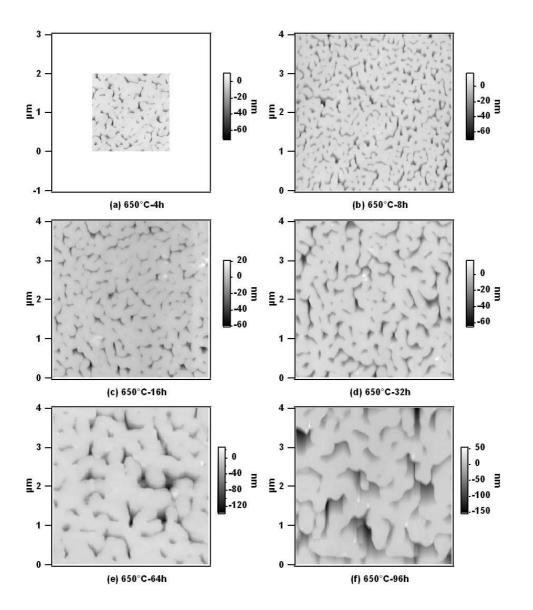
Fig. 1. AFM height images of borosilicate glass samples after thermal treatment at  $650^{\circ}\mathrm{C}$  during six different durations.
