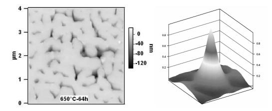
Fig. 4. AFM height images  $(4 \times 4\mu m^2)$  of a borosilicate glass sample after 64 hours of thermal treatment at 650°C (left) and the associated three dimensional representation of the center part  $(0.5 \times 0.5\mu m^2)$  of the auto-correlation function  $C(\vec{x})$ (right).
