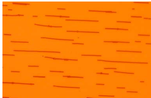
Figure 6. An example of the straight aggregates formed by 4 \mu\text{m} spheres in 10 Oe magnetic field after about 2 hours.
