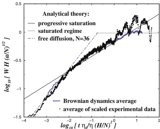
FIG. 2 (color online). Scaling of the random mean square width of the transverse displacements: theory, experiments, and Brownian dynamics result. The units are Oe,  $\mu\text{m}$ ,  $\mu\text{m}$ , and seconds for  $H$ ,  $a$ ,  $W$ , and  $t$ , respectively.
