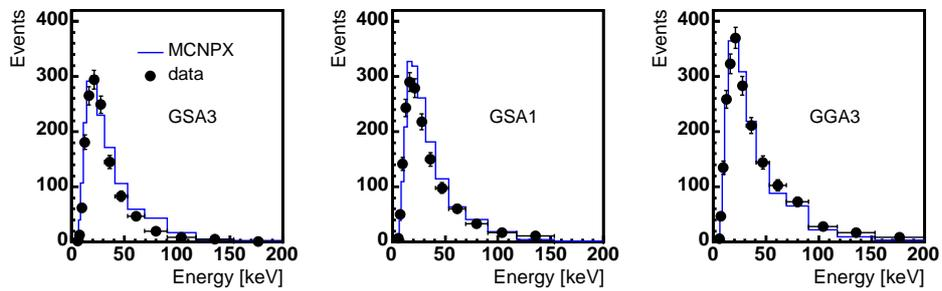
Figure 6: Energy spectra of the nuclear recoils in EDELWEISS-I calibration runs with a  $^{252}\text{Cf}$  neutron source. The MCNPX simulation is also shown (full line, no normalization to data).
