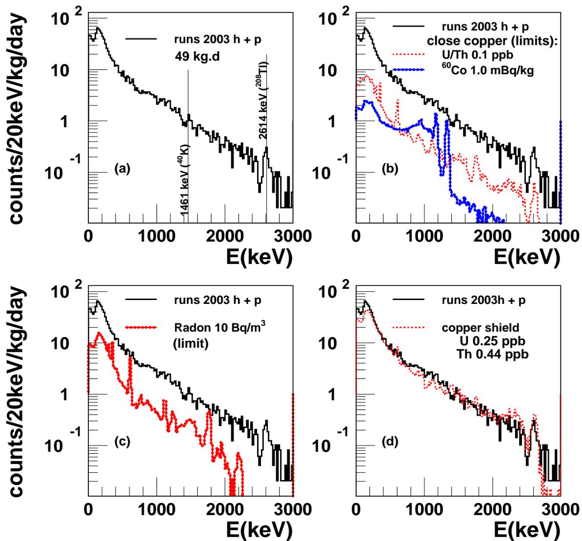
Figure 2: Gamma background energy spectrum (ionization channel) compared to Monte Carlo simulations of various sources of radioactive contamination (see text). The sum of the 2003p and 2003h data sets is shown, for the total volume of the three detectors (49 kg.d).
