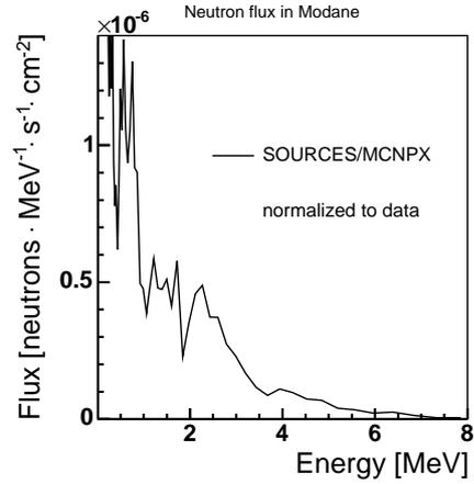
Figure 8: Simulated neutron energy spectrum in the LSM after normalization to data. The neutron production from  $^{238}\text{U}$  and  $^{232}\text{Th}$  traces in the rock is simulated with SOURCES and propagated with MCNPX.
