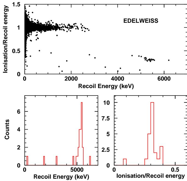
Figure 3: Distribution of the ionization quenching ratio  $Q$  with recoil energy  $E_R$ , for the data of the run 2003h. Bottom left:  $E_R$  projection for  $0.2 < Q < 0.4$ . Bottom right:  $Q$  projection for  $4.5 < E_R < 6$  MeV.
