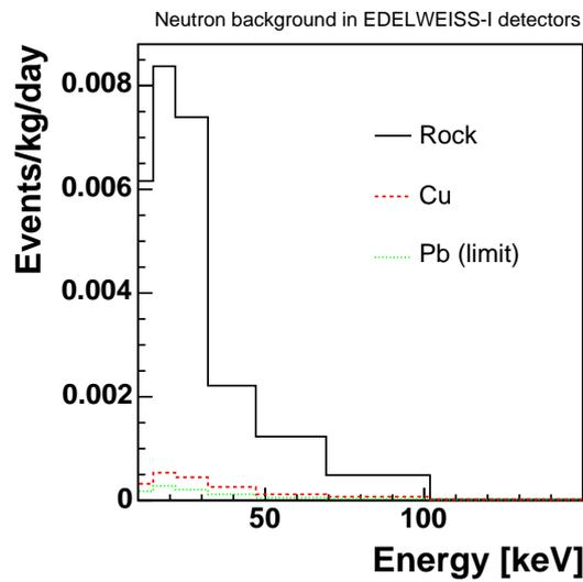
Figure 9: Expected energy spectra of the nuclear recoils in EDELWEISS-I low-background runs from radioactivity of the rock (full line),  $^{238}\text{U}$  contamination in copper (dashed line) and in lead (dotted line).
