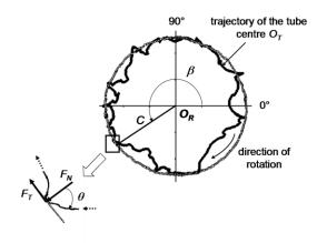
Figure 2. Motion of the tube specimen in the ring, represented by the trajectory of the tube centre  $O_T$  in the tube-ring clearance represented by a circle of radius *C* and centre  $O_R$ . A sliding impact is
