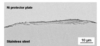
Figure 10. SEM observation of a cross section of worn surface of specimen L2.
