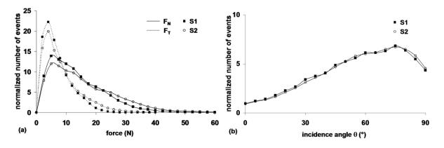
Figure 4. Comparison of (a) force histogram and (b) incidence angle histogram for wear tests S1 and S2.
