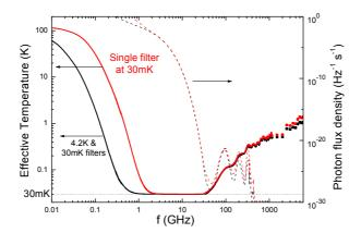
Calculated effective temperature (full lines, left axis) seen by a device connected to a line comprising a 50  $\Omega$  source at 300 K and either a single filter (red curves) anchored at 30 mK or two filters (black curves) respectively placed at 4.2 K and 30 mK and photon flux density (dashed lines, right axis) at the output of this line on a 50  $\Omega$  load.
