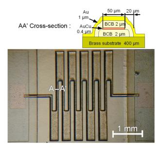
Picture of a microfabricated filter chip, and cross-section of a meander arm with materials and respective thickness (note different vertical and horizontal scales).
