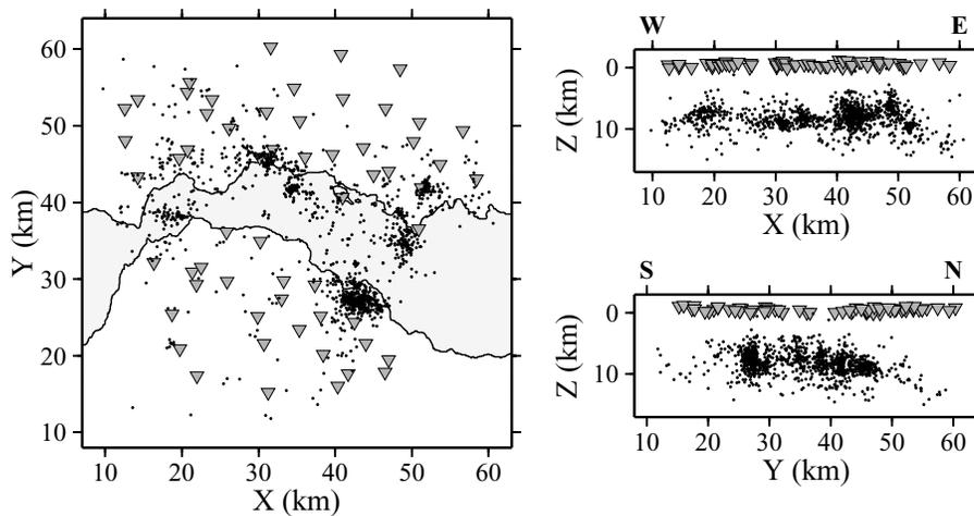
**Figure 2.** The right panel shows the area where the temporary network of seismic stations (inverted triangles) was deployed during the 1991 seismic experiment. Earthquake hypocentres (dark dots) have been located using the HYPO71 procedure. Right panels show the W–E (top) and S–N (bottom) cross-sections of the investigated area. Earthquakes and stations are projected on these sections.
