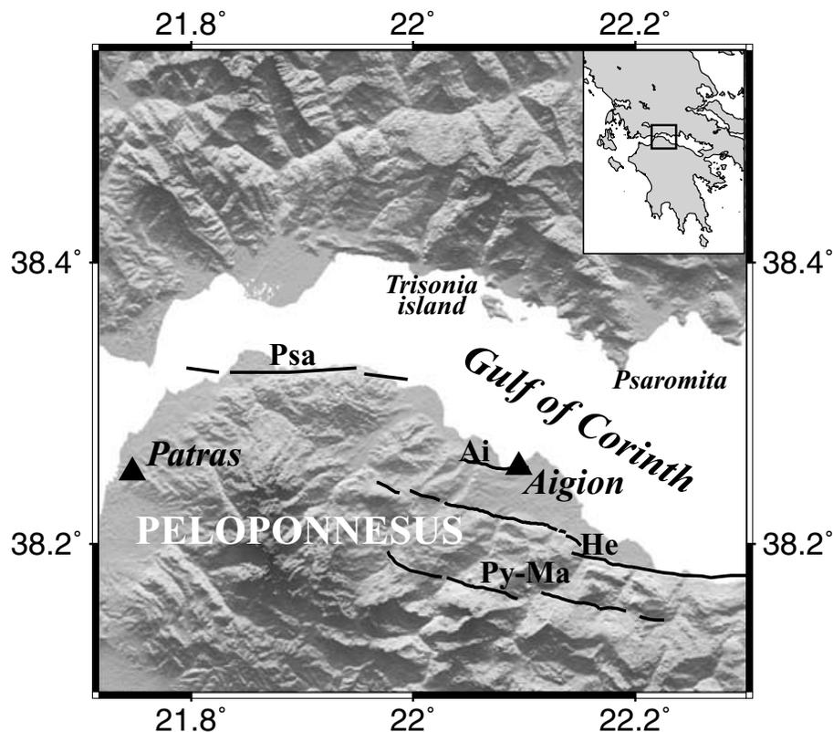
**Figure 1.** Map of the western Gulf of Corinth. The location of the selected area is indicated on the right corner of the figure. The major north-dipping normal faults cropping out in the Peloponnesus are represented by dark lines. Psathopyrgos fault (Psa), Aigion fault (Ai), Helike fault (He), Pyrgaki–Mamoussia fault (Py–Ma).
