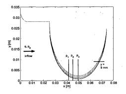
Fig. 1. Pharyngeal geometry represented by a flat bottom plate corresponding to y=0 and demi-cylinders with diameter d=49mm for the assessed  $h_{min}$ 's (0.70, 1.00, 1.45, 1.90 and 2.30mm). The y-axis corresponds with the distance between the flat plate and the demi-cylinder. The x-axis presents the distance along the longitudinal axis of the replica. The sensor sites are indicated with a solid blue line.
