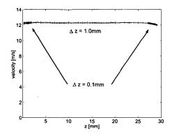
Fig. 2. Horizontal velocity profile (0 up to 30mm and 30 down to 0mm) for  $h_m in = 2.3mm$  and a steady flow of 60 Vmin.
