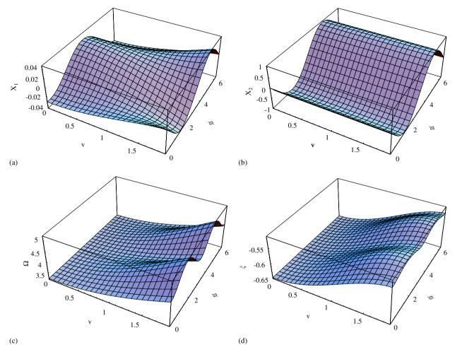
Fig. 5. Nonlinear mode which coincides for small values of v with the second mode of the underlying linear system of the dissipative system with non-proportional damping: (a)  $X_1$  versus v and  $\phi$ , (b)  $X_2$  versus v and  $\phi$ , (c)  $\Omega$  versus v and  $\phi$  and (d)  $\xi$  versus v and  $\phi$ .
