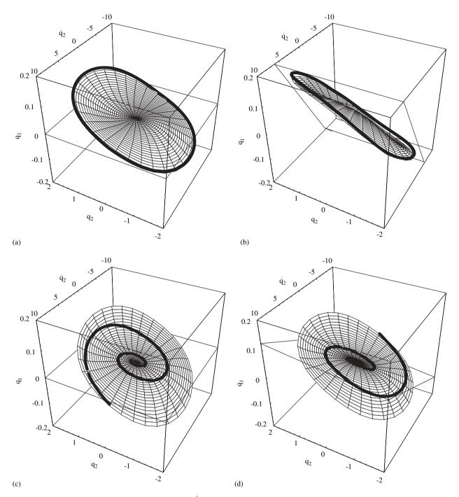
Fig. 6. Invariant manifold in the phase subspace  $(Q_1, Q_2, \dot{Q}_2)$ : (a) non-gyroscopic conservative system, (b) gyroscopic conservative system, (c) proportional damping and (d) non-proportional damping.
