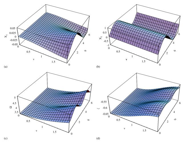
Fig. 4. Nonlinear mode which coincides for small values of v with the second mode of the underlying linear system of the dissipative system with proportional damping: (a)  $X_1$  versus v and  $\phi$ , (b)  $X_2$  versus v and  $\phi$ , (c)  $\Omega$  versus v and  $\phi$  and (d)  $\xi$  versus v and  $\phi$ .
