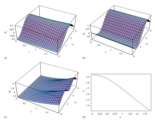
Fig. 3. Nonlinear mode which coincides for small values of v with the second mode of the underlying linear system of the gyroscopic conservative system: (a)  $X_1$  versus v and  $\phi$ , (b)  $X_2$  versus v and  $\phi$ , (c)  $\Omega$  versus v and  $\phi$  and (d) period versus a.
