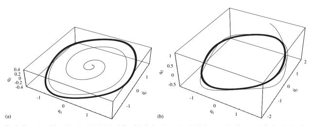
Fig. 9. Illustration of the (a) local and (b) global stability of the limit cycle associated with the second nonlinear mode: limit cycle given by  $v_2^*$  (bold continuous lines), motions obtained by solving Eq. (68) with initial conditions inside the invariant manifold (a) (continuous line) and outside the invariant manifold (b) (continuous line).
