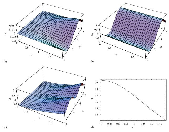
Fig. 2. Nonlinear mode which coincides for small values of v with the second mode of the underlying linear system of the non-gyroscopic conservative system: (a)  $X_1$  versus v and  $\phi$ , (b)  $X_2$  versus v and  $\phi$ , (c)  $\Omega$  versus v and  $\phi$  and (d) period versus a.
