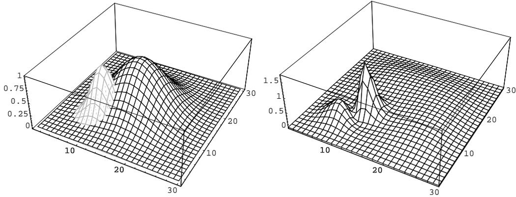
Fig. 1. Left : laser beam Gaussian profile to be coupled in the waveguide (black) and waveguide (grey) (A.U.). Right : beam profile after a 3mm propagation. The window size is  $30\mu\text{m}$  and the beam wavelength is  $250\mu\text{m}$ . The highest peak on the right evidences the light which is coupled into the waveguide.
