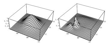
FIG. 1: Left: laser beam Gaussian profile to be coupled in the waveguide (A.U.). Right: beam profile after a 3mm propagation. The window size is  $30\mu m$  and the beam wavelength is  $250\mu m$ . The highest peak on the right evidences the light which is coupled into the waveguide.
