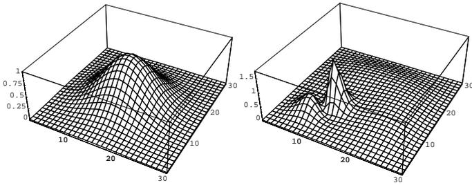
FIG. 1: Left : laser beam Gaussian profile to be coupled in the waveguide (A.U.). Right : beam profile after a 3mm propagation. The window size is  $30\mu\text{m}$  and the beam wavelength is  $250\mu\text{m}$ . The highest peak on the right evidences the light which is coupled into the waveguide.
