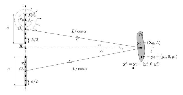
Figure 7: Symmetric geometry setup for distributed reflectivity imaging.
