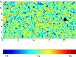
Figure 4: A typical realization of the random sound speed  $c(\mathbf{x})$ . The target is shown as a large black dot  $\bullet$ . The units in the horizontal and vertical axes are mm and, in the color bar, km/s. The standard deviation for this example is s = 4.95%
