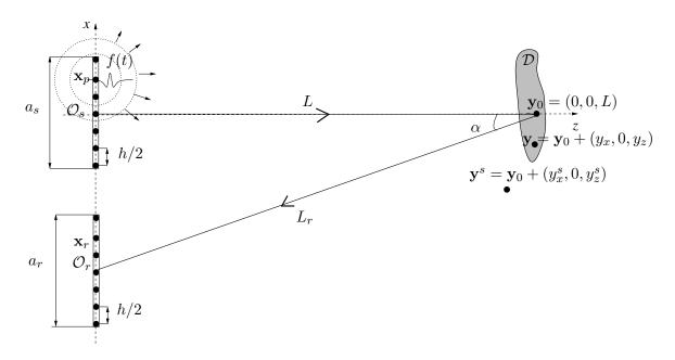
Figure 6: The setup for distributed reflectivity imaging.
