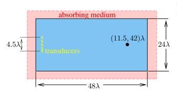
Figure 3: The computational setup. The dimensions of the problem are given in terms of the central wavelength  $\lambda = 0.5$ mm. The medium is considered to be infinite in all directions so in the numerical computations an absorbing layer surrounds the domain.
