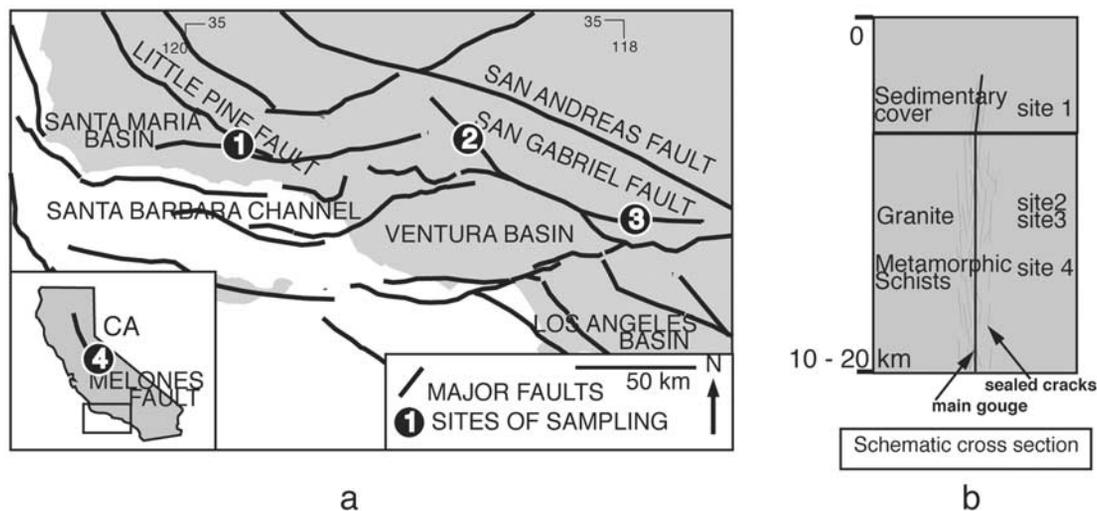
**Figure 2.** (a) Schematic map indicating the locations of the sampling sites: site 1, Little Pine fault; sites 2 and 3, San Gabriel fault; site 4, Melones fault (Mother Lode valley). Fault map of the Transverse Ranges Province adapted from *Jennings* [1994]. (b) Schematic cross section of a synthetic California strike slip fault affecting the entire seismic crust, with indication of the level of the various sampling sites.
