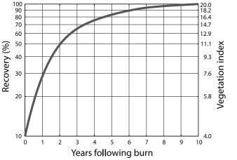
**Figure A1.** Vegetation growth recovery from *LACFCD* [1959]. After 10 years, bush vegetation has almost fully recovered from former fires. In our computation we assume that the vegetation index (Ve in equation (2)) varies in proportion with the growth recovery and reaches a value Ve = 20 after 10-12 years, when growth recovery is complete.
