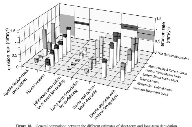
**Figure 18.** General comparison between the different estimates of short-term and long-term denudation rates in the five different morphotectonic units defined in the San Gabriel Mountains. Note that by contrast with Figures 5 and 8, average sediment production rates are volumetric averages.
