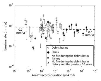
**Figure 8.** Computed erosion rates (mm yr<sup>-1</sup>) for debris basins (gray circles) and dams (black circles) after subtraction of the contribution due to fire effects. After correction, data scatter for the debris basins has been reduced but remains significant. The average value for small watersheds, however, is now only 25% more than denudation values recorded in dams.
