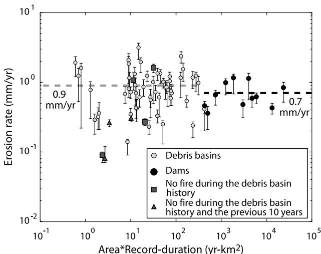
**Figure 8.** Computed erosion rates ( $\text{mm yr}^{-1}$ ) for debris basins (gray circles) and dams (black circles) after subtraction of the contribution due to fire effects. After correction, data scatter for the debris basins has been reduced but remains significant. The average value for small watersheds, however, is now only 25% more than denudation values recorded in dams.
