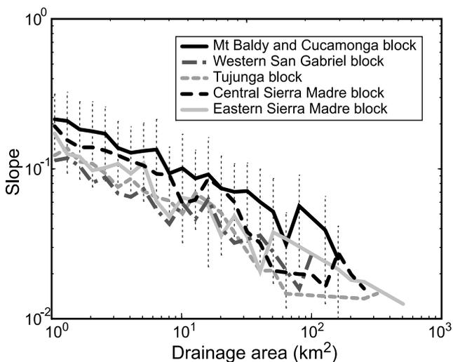
**Figure 14.** Slope-area relationship for the San Gabriel Mountains. For drainage areas  $>1 \text{ km}^2$ , the average curvature ( $-m/n$ ) ratios range between  $-0.37$  and  $-0.43$  for the five morphotectonic regions, as expected from a shear stress or unit stream power model for fluvial incision. Vertical dashed lines represent the  $1\text{-}\sigma$  uncertainties on the Mount Baldy-Cucamonga region mean slopes.
