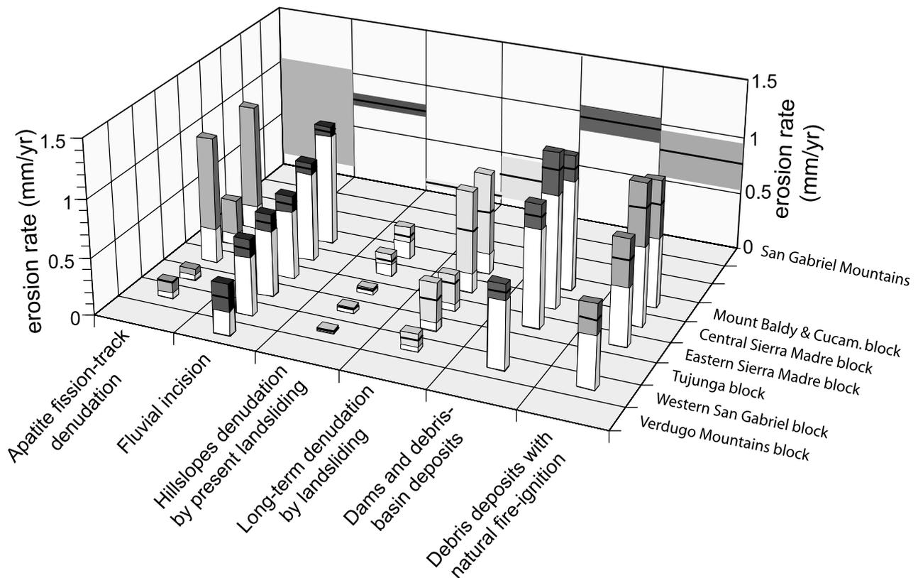
**Figure 18.** General comparison between the different estimates of short-term and long-term denudation rates in the five different morphotectonic units defined in the San Gabriel Mountains. Note that by contrast with Figures 5 and 8, average sediment production rates are volumetric averages.
