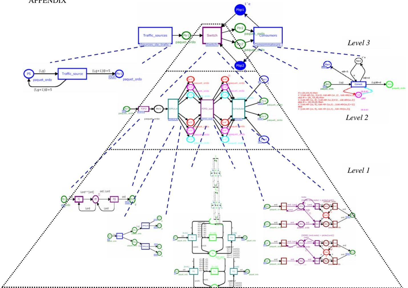
Fig. 2. Hierarchical model of Ethernet switch
