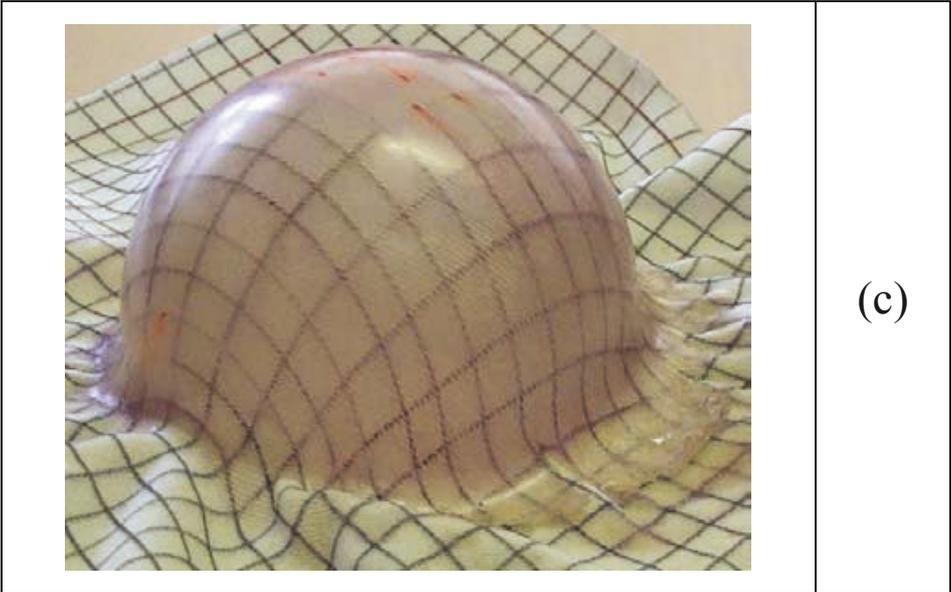
**Figure 5.** *Shape of the unbalanced fabric after forming*
