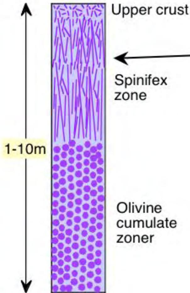
The cooling rate 2 m beneath the top of a komatiite flow should be low ( $\sim 1-5^{\circ}\text{C/h}$ ), but the dendritic morphologies of olivine crystals in spinifex textures resemble those of crystals that form at high cooling rates in dynamic crystallisation experiments
