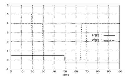
Figure 1: Known input u(t) and unknown input d(t).
