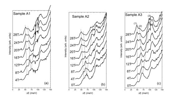
**Fig. 1** Magneto-PLE spectra of samples A1 (a), A2 (b) and A3 (c) at 4 K from B=0 to B=28 T every 4 T and for a  $E_{det}=1215$  meV. The dashed lines are guides for the eyes. Traces have been vertically offset for clarity.
