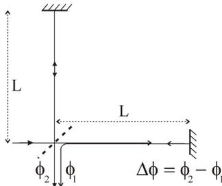
Fig. 2. Michelson interferometer.
