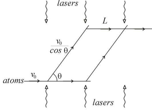
Fig. 5. Ramsey-Bordé interferometer in the  $X$ - $Y$  plane.
