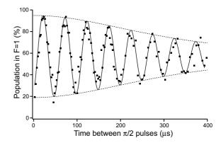
FIG. 3: Ramsey fringes recorded with a  $\pi/2$  pulse length of 1.2  $\mu$ s and a detuning  $\delta = 2\pi \times 20.8$  kHz. The solid line is a fit to the data using the model presented in [18], which yields a dephasing time  $T_2^* = 370~\mu$ s.
