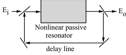
Fig. 1. Ikeda considered the case of a nonlinear passive cavity located in a ring resonator and modeled by a delay differential equation (DDE).  $E_i$  and  $E_o$  are the amplitudes of the injected and output fields, respectively. The delay is the round-trip time along the optical-path.
