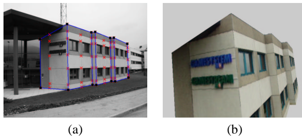
Figure 1. Example of piecewise planar modeling: (a) shows an image overlaid with the automatically recovered piecewise planarity and (b) the model rendered from a different point of view.
