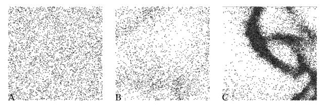
FIG. 3: Three snapshots of a small part of the gas of  $10^6$  inelastic hard disks with restitution coefficient  $\alpha=0.9$ . In the snapshots is portrayed a square of surface  $200\times200$ , in units of a diameter, where the whole system is  $3163\times3163$ ; therefore the pictures portray a fraction 0.004 of the total surface. **A**: just after thermalization (0 collisions per particle (cpp)). **B**: after 100 cpp (collisions per particle). **C**: after 200 cpp.
