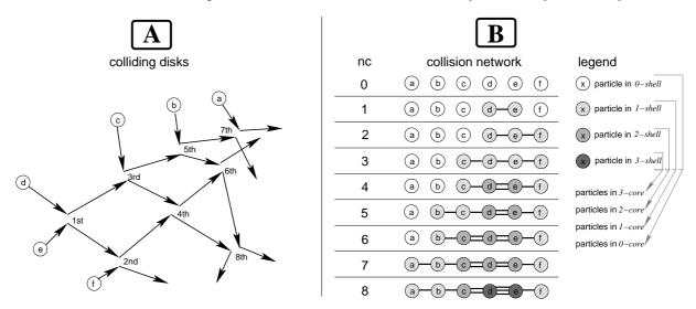
FIG. 1: Evolution of the network of collisions for a system of 6 particles. A: the ordered sequence of collisions. B: collision network at each time step, where nc is the number of realized collisions. All particles are in core of index 0. Particles not appearing in higher cores are also in shell of index 0. In general a k-core has all the particles with shell index  $\geq k$ .
