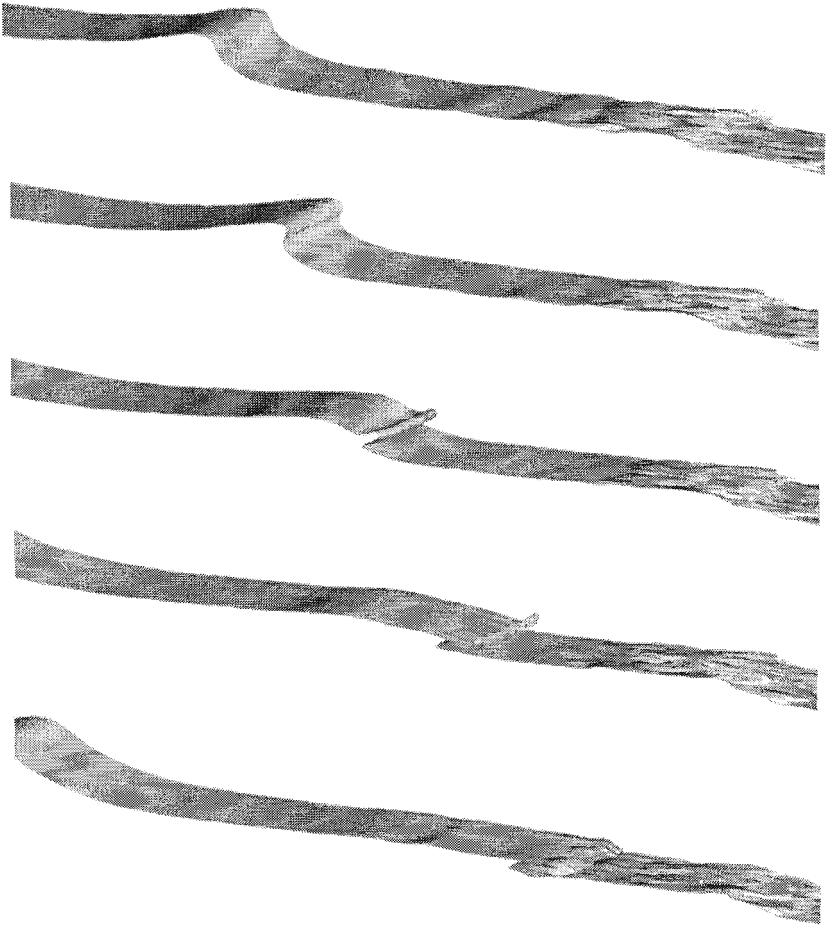
Figure 8. Numerical results for 3D waves breaking (14 th wave). Color function C = 0.5 .
