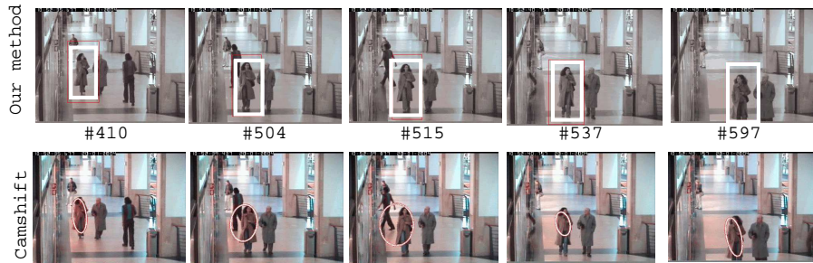
Fig. 7. Example of pedestrian tracking (The video sequence comes from Caviar database. Upper images show results obtained for the tracker and lower images show results obtained for the CAMSHIFT Tracker
