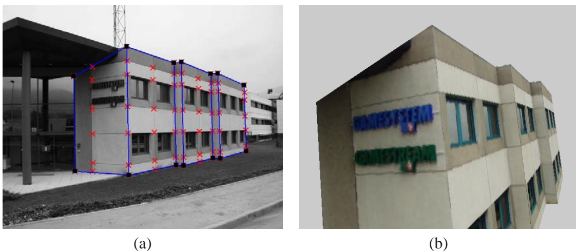
Figure 1: Example of piecewise planar modeling: (a) shows an image overlaid with the automatically recovered piecewise planarity and (b) the model rendered from a different point of view. The reconstruction process for this example is detailed in §6.2.2.
