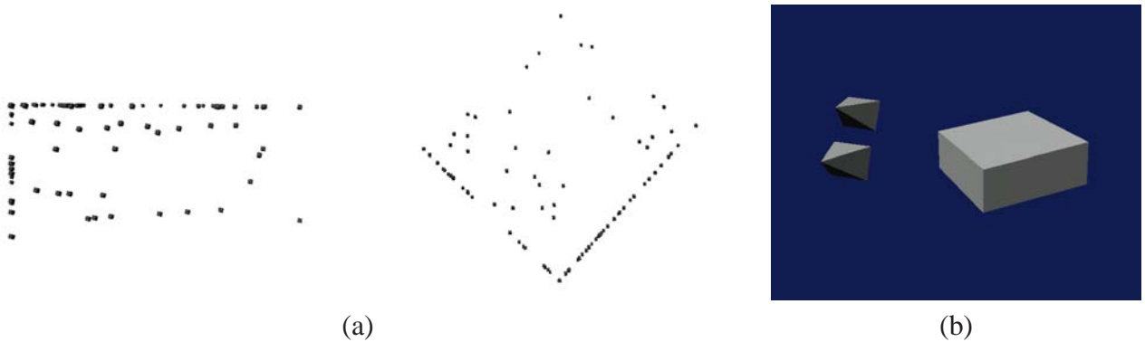
Figure 11: Piecewise planar model obtained for the BOX dataset. (a) shows the sparse point reconstruction constrained by the planes, and (b) shows the model consisting of three planes and two cameras. We observe on (a) that the reconstructed points are perfectly coplanar after constrained bundle adjustment.
