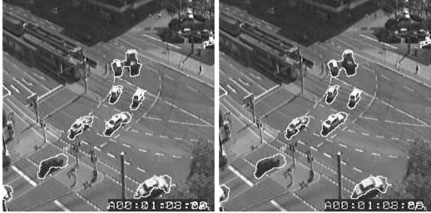
Figure 2: Results obtained (10th image of the sequence) with TV_{1,g} and TV_{1,g,\frac{\pi}{4}} and the optical flow norm as initial data. Parameters are \alpha = 0.6 , \lambda = 0.2 and \mu = 10 . Notice the smoothness of the result on the right image in comparison to the one on the left image.
