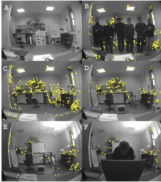
Figure 10: Images for robustness evaluation on axis : original image (A), occultation by 6 persons (B), modifications step 2 (C), step 4 (D), step 6 (E) and step 8 (F)
