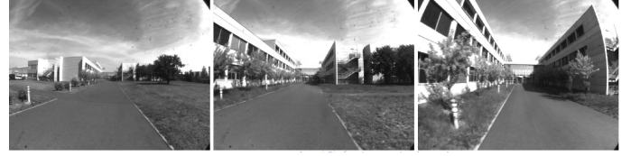
Fig. 4. Principle of vision based localization. 1) vehicle freely moves and records a video sequence. 2) trajectory and visual features of the video are reconstructed. 3) vehicle can localize itself and take the same path.
