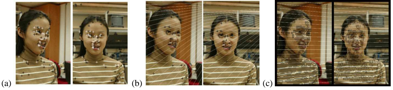
Figure 4: (a) Initial sparse correspondences by cross-correlation for a pair of images with large disparities. Only 31 matches in white out of 111 are correct. (b) Failure of the standard sparse method. Many correspondence points in black are obviously incorrect. (c) Successful quasi-dense estimation.
