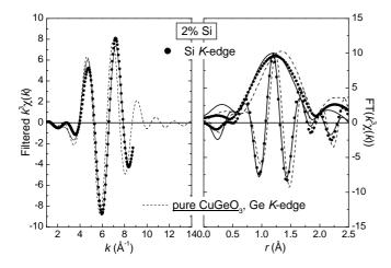
**Fig. 8.** EXAFS results for 2% Si-doped CuGeO<sub>3</sub>. Amplitude and imaginary part of the FT of  $k^3\chi(k)$  (right) and Fourier filtered  $k^3\chi(k)$  (left) at the Si K-edge of the doped sample (full circles) compared to the fit (solid lines) and to the results obtained at the Ge K-edge on the pure sample (dashed lines).
