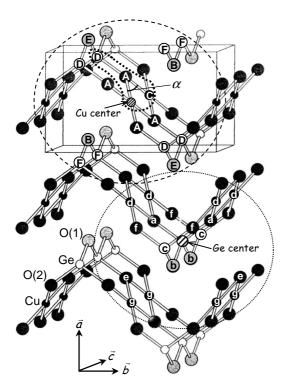
Fig. 4. Structure of CuGeO<sub>3</sub>. The Cu and Ge environments are materialized: starting from the dashed Cu and Ge absorbers, the atoms labelled "A", "B", ... "F" (for Cu) and "a", "b", ... "g" (for Ge) are their neighbors going from the closest to the furthest ones that were accessible in the EXAFS experiment.
