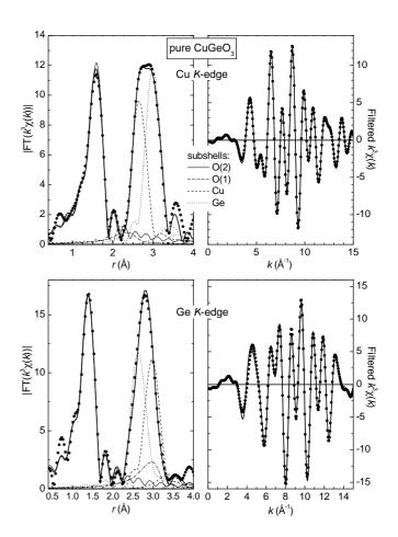
**Fig. 5.** EXAFS results for the pure  $CuGeO_3$  sample. Amplitude of the FT of  $k^3\chi(k)$  (left) and Fourier filtered  $k^3\chi(k)$  (right) at the Cu (top) and Ge (bottom) K-edges. The measured spectra are represented by full circles, the fit by a thick solid line. The contributions of each kind of neighbors are also shown on the FT plots (left).
