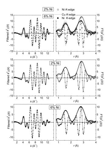
**Fig. 6.** EXAFS results for the 2% and 6% Ni-doped CuGeO<sub>3</sub>. Amplitude and imaginary part of the FT of  $k^3\chi(k)$  (right) and Fourier filtered  $k^3\chi(k)$  (left). Comparison of the measured spectra at the Ni K-edge for both doping levels and at the Cu K-edge for 6% Ni sample (top). Comparison of the measured spectra (circles) and of the fits (solid lines) at the Ni K-edge for 2% doping (middle) and 6% doping (bottom).
