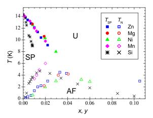
**Fig. 2.** (Temperature - concentration) magnetic phase diagram for  $\text{CuGe}_{1-x}\text{Si}_x\text{O}_3$  and  $\text{Cu}_{1-y}M_y\text{GeO}_3$ , with M=Zn, Mg, Ni, and Mn.
