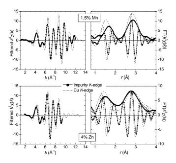
**Fig. 7.** EXAFS results for 1.5% Mn (top) and 4% Zn (bottom) doped CuGeO<sub>3</sub>: amplitude and imaginary parts of the FT of  $k^3\chi(k)$  (right) and Fourier filtered  $k^3\chi(k)$  (left) of the measured data (full circles) and their fits (solid lines) at the impurity K-edge. The Cu K-edge spectra measured on the same sample are also shown (dashed lines), for comparison.
