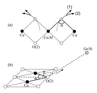
**Fig. 9.** Schematic view of the local deformation, due to  $M/\mathrm{Cu}$  (a) and Si/Ge (b) substitution, assumed for the calculation of the local Cu(or M)-O(2)-Cu angle  $\alpha$  (see text for the different scenarii).
