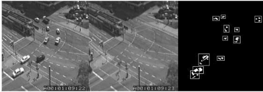
Figure 4 : Smart camera executing. Left: video from the camera, center: background detection, right: moving objects detection
