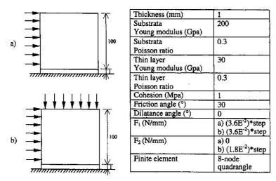
Fig. 2 The first two examples: a bar bonded with a plane (the dimensions are in mm)
