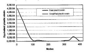
Fig. 9 Equivalent plastic strain along the substratum/thin layer interface: example 3 at step 50
