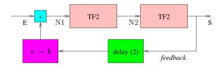
Each TF2 element itself a complex filter with internal filter feedback loop.
