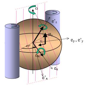
FIGURE 10. Schematic representation of the distorted magnetic field lines associated with the  $\Omega$  effect generated by the spin-over mode of the elliptical instability in the rotating deformed sphere.
