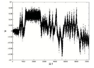
FIGURE 1. Doppler anemometry measurements of the radial velocity somewhere in the rotating deformed cylinder. Intermittent cycle of elliptical instability in the cylinder (where the phase of the unstable mode changes between two cycles) would imply a reversal of the magnetic field in MHD; one can also notice that the characteristic times of the dynamics range from the rotation period to thousands of rotation periods.
