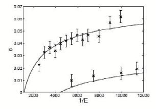
FIGURE 5. Comparison between the linear analysis of elliptical instability in the sphere and experimental measurements of the growth rates  $\sigma$  of the spin-over for two cases of ellipticity ( $\epsilon = 0.08$  and 0.16).
