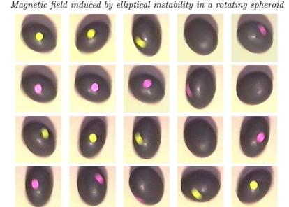
FIGURE 4. Series of chronological images showing two heteroclinic cycles of the axis of rotation of the elliptical spinning top.
