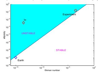
FIGURE 6. Stability of a flow in a sphere in the presence of an elliptical deformation, depending on the Ekman number and on the imposed ellipticity. Data for Io come from Kerswell and Malkus (1998) and are derived from Anderson *et al.* (1996). The straight line is given by  $\sigma = 0$  (see equation 1.1)
