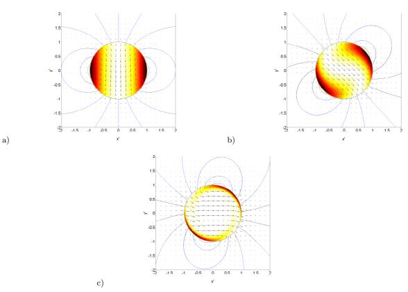
FIGURE 8. Arrows represent the induced magnetic field in the (tilted) equatorial plane ( $\theta' = \pi/2$ ). Field lines outside the sphere are solid lines. Joule dissipation  $|\nabla \times \mathbf{H}'|^2$  inside the sphere is indicated by the gray scale. (a)  $Re'_m = 0.01$ , (b)  $Re'_m = 10$ , (c)  $Re'_m = 100$ . Note that the field is perpendicular to the spin-over axis at low  $Re'_m$  but tends to be parallel at higher  $Re'_m$ .
