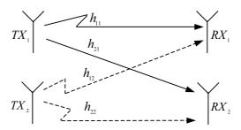
Figure 2. Channel Model for MIMO  $2 \times 2$
