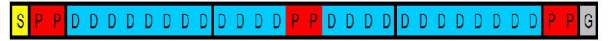
(c) Downlink frame: S = synchronization, G = Guard, P = Pilot, and D = data OFDM symbol
