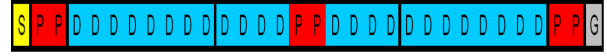
(c) Downlink frame: S = synchronization, P = pilot, G = guard, and D = data OFDM symbol
